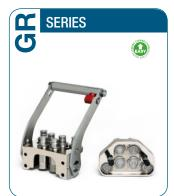
Valving style: Flat face Interchange: Stucchi interface Available sizes: From 3/8" to 1" Operating pressure: Up to 350 bar Flow rate: Up to 378 L/Min Material: Brass & high strength carbon steel
