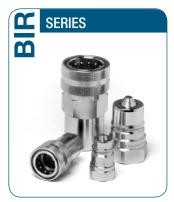
Valving style: Poppet Interchange: ISO 7241-1 "A" Available sizes: From 1/4" to 2" Operating pressure: Up to 350 bar Flow rate: **Up to 1000 L/Min** Material/treatment: Carbon steel/Cr3 Connection system:
