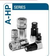
Valving style: Flat face Interchange: Stucchi profile Available sizes: From 1/8" to 3/8" Operating pressure: Up to 720 bar Flow rate: Up to 46 L/Min Material/treatment: Carbon steel/Cr3 Connection system: Push Connection under pressure:
