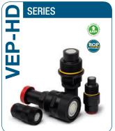
Valving style: Flat face Interchange: Stucchi profile Available sizes: From 3/4" to 1-1/2" Operating pressure: Up to 550 bar Flow rate: Up to 750 L/Min Material: Carbon steel/QPQ Connection system: Screw Connection under pressure:
