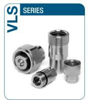
Valving style: Poppet Interchange: Similar Couplings Available sizes: From 1/2" to 1" Operating pressure: Up to 465 bar Flow rate: Up to 200 L/Min Material/treatment: Carbon steel/Cr3 Connection system: Screw
