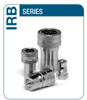
Valving style: Poppet Interchange: ISO 7241-1 "B" Available sizes: From 1/8" to 1" Operating pressure: Up to 350 bar Flow rate: **Up to 200 L/Min** Material/treatment: Carbon steel/Cr3 Connection system:
