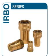
Valving style: Poppet Interchange: ISO 7241-1 "B" Available sizes: From 1/8" to 1" Operating pressure: **Up to 200 bar** Flow rate: **Up to 200 L/Min** Material: Brass Connection system: Single acting sleeve Connection under pressure: Not allowed
