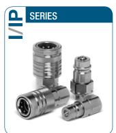
Valving style: Poppet Interchange: ISO 7241-1 "A" Available sizes: From 1/4" to 1" Configuration: Modular construction Operating pressure: Up to 350 bar Flow rate: Up to 200 L/Min Material/treatment: Carbon steel/Cr3 Connection system: Push-pull Connection under pressure: Not allowed
