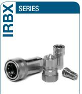
Valving style: Poppet Interchange: ISO 7241-1 "B" Available sizes: From 1/8" to 1" Operating pressure: Up to 250 bar Flow rate: Up to 200 L/Min Material: Stainless steel (AISI 316L) Retainer in brass Connection system: Single acting sleeve Connection under pressure: Not allowed
